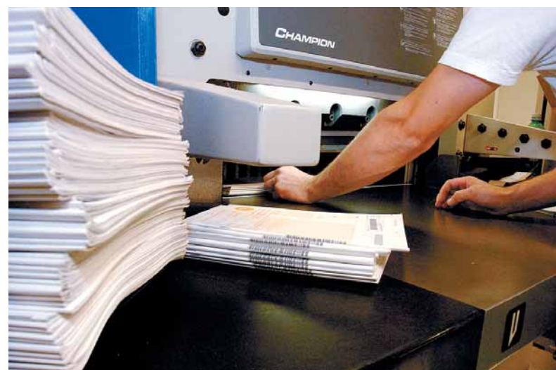
A worker inserts bundles of tests into a binding-removal machine.
